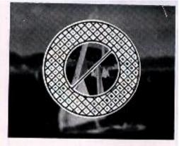
Look through the viewfinder to compose your picture and focus by turning the Focusing Ring. You can focus either by using the center Split-image Spot or the Microprism Image Band that surrounds the center circle.
